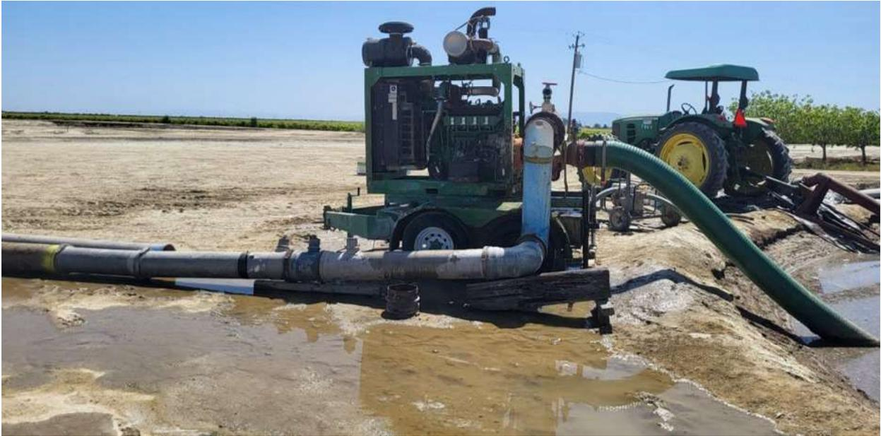
Water is being pumped using diesel power take-off (PTO) motors from the basins into the pistachio orchards and wine-grape vineyards using thousands of feet of pipe across the entire ranch to convey water to different plantings for on-farm recharge.
